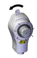
Hold the quick-prime key firmly in place and slide it fully to the left. The pusher will release to the max 30ml dose position, to enable the unit to be primed
