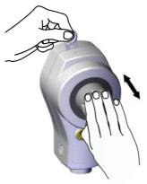
Continue to hold the quick-prime key in place. Repeatedly press the pusher to prime the unit
