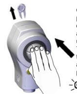
Once the unit is fully primed, remove the quick-prime key and press the pusher until you hear a click. The unit is now ready to operate normally at its original dose position
